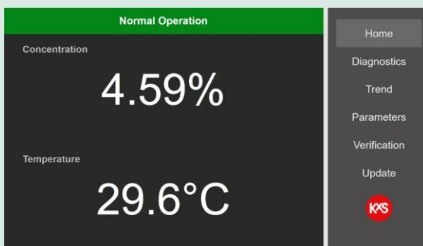
However, external displays with different sizes are available for connection through the sensor digital port. Computer, tablet or mobile phone with a web browser serves as user interface for accessing sensor diagnostics and settings.
