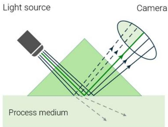
This interface is detected by the light-activated camera pixels and converted into refractive index (RI).
