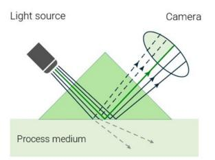
This interface is detected by the lightactivated camera pixels and converted into refractive index (RI).
