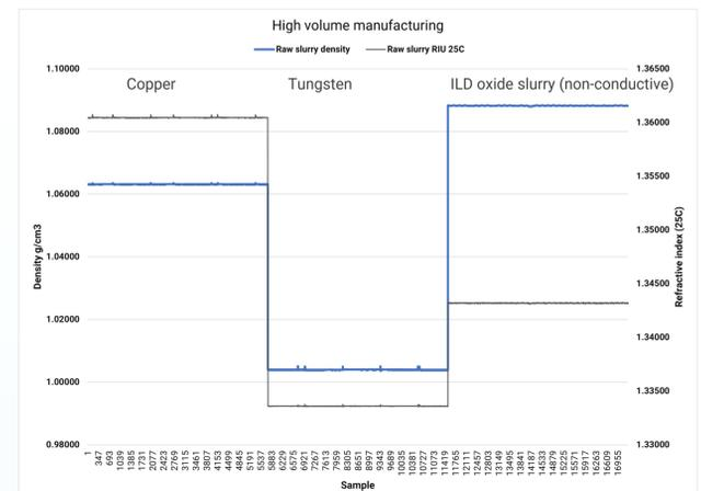
It is known that slurry batches as delivered by the vendor present a density range. As shown in the upper chart, respective slurry type has its typical density level. The middle chart again shows that for the ILD oxide slurry, **inline RIU detects UPW %m/m additions** with an approximate **Limit of Detection LOD = 0.051**, while an **inline densitometer** with an approximate **LOD = 0.074** (lower is better).
