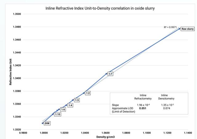
In the wafer edge polishing process, the measurement signal confirmed the slurry:UPW ratio going to the polisher repeatable. Further work will focus on defining a process control function to achieve and ensure a stable slurry ratio at target level.
